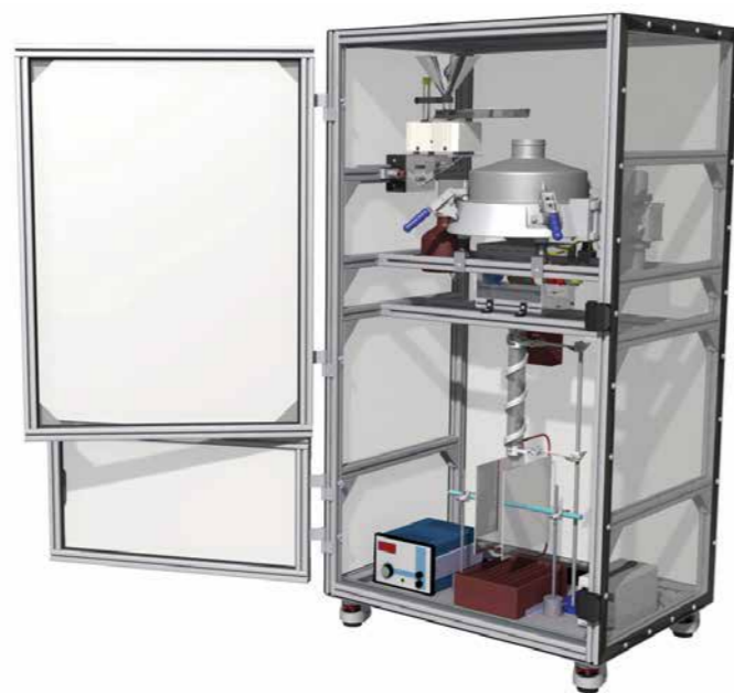
CAD model of the multi-stage Regolith beneficiation experiment
