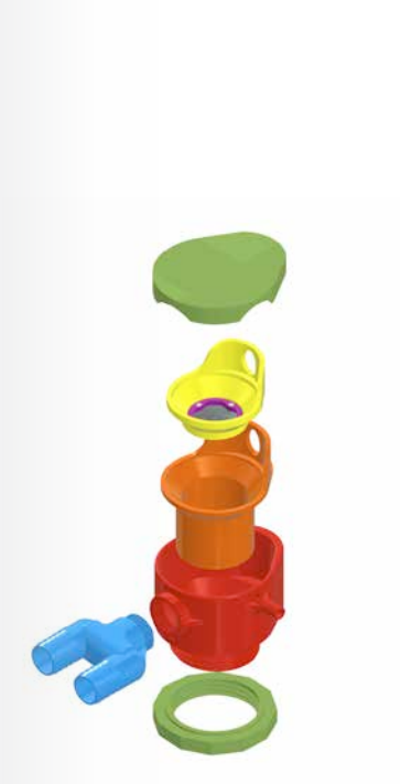
Explosion view of the adapter between the seed cultivation mats and the MEPA support unit
