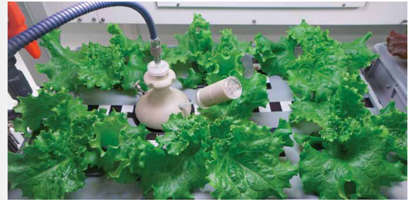
The E-nose system being used to detect contamination of leafy greens
