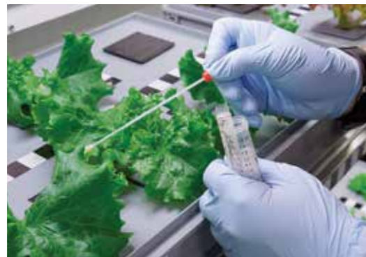
Taking microbial samples of leafy greens as part of the EDEN ISS sample return mission
