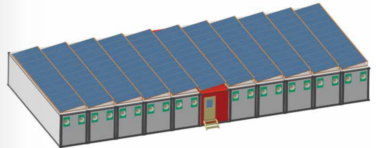
Initial CAD model of a modular closed-loop arid greenhouse system developed during the PMARS and GERF design study
