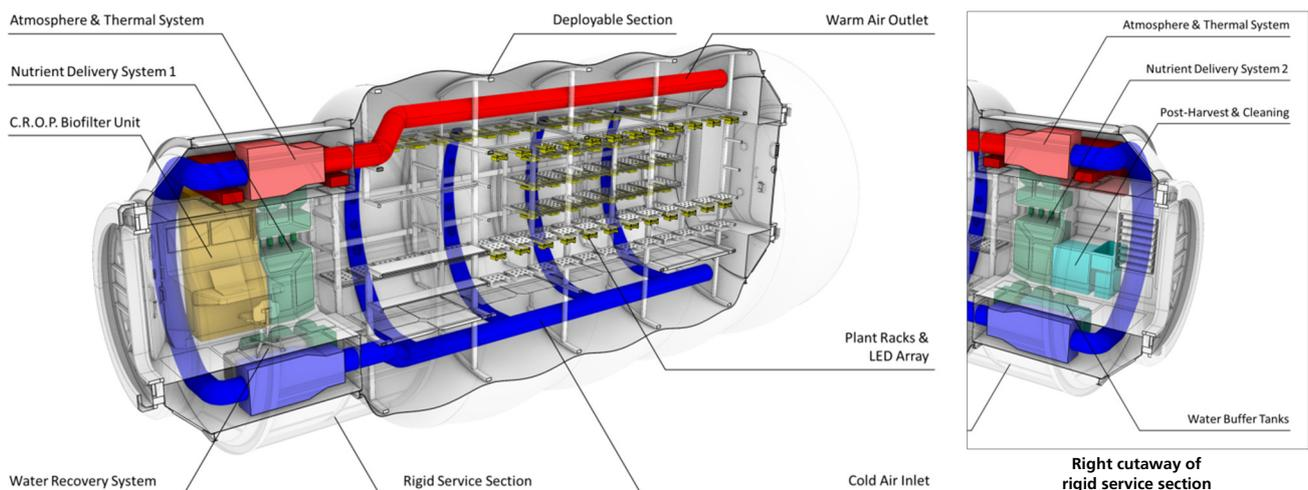
Figure 3: Left and right cutaway of the DLR BLSS test demonstrator.
