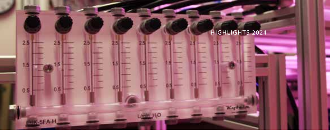
Adjustable nutrient solution flow distribution ensuring equal delivery to each channel.
