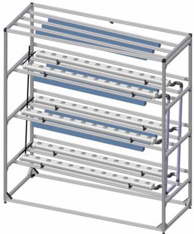
CAD model of the BioLoops production rack.
