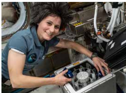
Fig. 2: Samantha Cristoforetti integrating a BIOFILMS experiment container (blue) into Kubik. The outer positions in Kubik allow incubation in microgravity. In the position inside the rotor in the middle, centrifugation is used to set different gravitational conditions. BIOFILMS samples were incubated at 20 °C for 14 days at \mu g , 0.4 \times g and 1 \times g in cubes. Image copyright: ESA.
