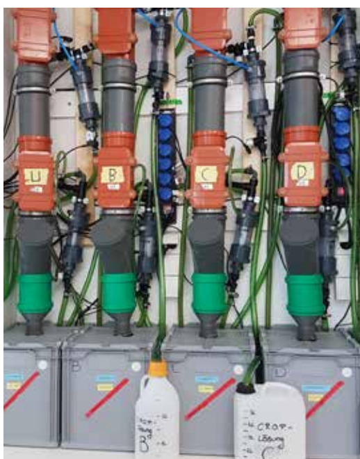
Fig. 1: The four C.R.O.P. ® -biofilters used in the experiment. The tubes contain lava rock as growth media. The grey tanks contain the urine solution. A pump circulates the solution continuously through the tubes thus bringing it repeatedly in contact with the biofilm in which nitrifying bacteria produce nitrate from the nitrogen compounds contained in the urine.
