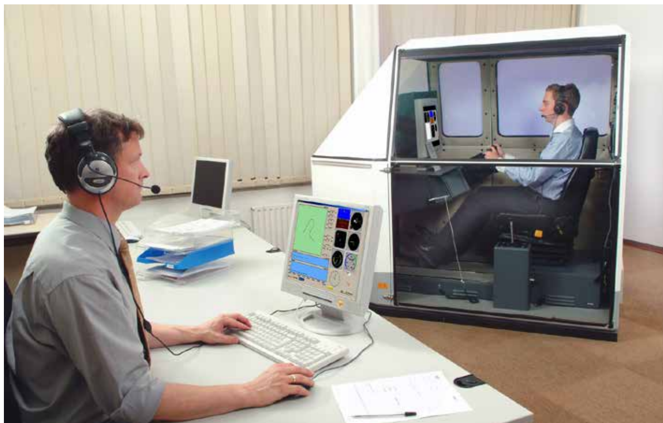
Fig. 1: The setup of the SIM with the test monitor in the foreground and the candidate in the back inside the test booth.
