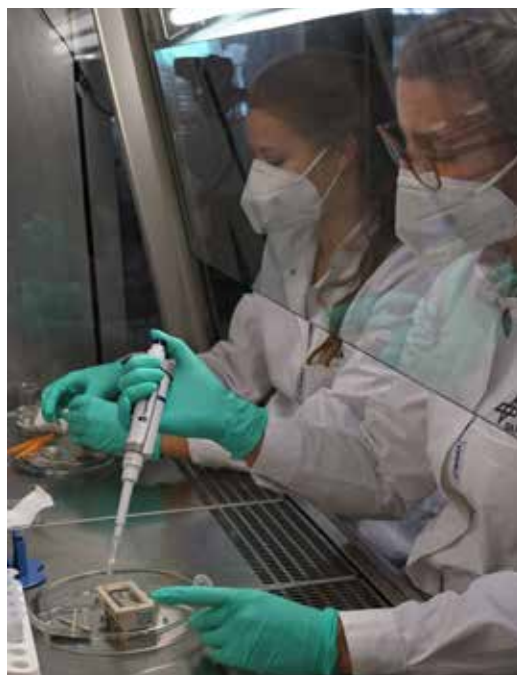
Fig. 1: Aerospace Microbiology Team during the disassembly of the experiment units from the second BIOFILMS mission. An experiment unit contained five metal surfaces (in the case shown in the picture, polished stainless steel). Before the surfaces can be removed, the liquid is pipetted off and transferred to reaction tubes for later analysis.
