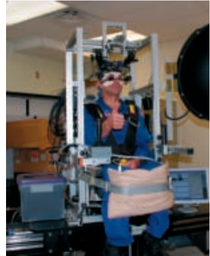
Astronauten testen die OTOLITH-Experimentalanlage in Houston
