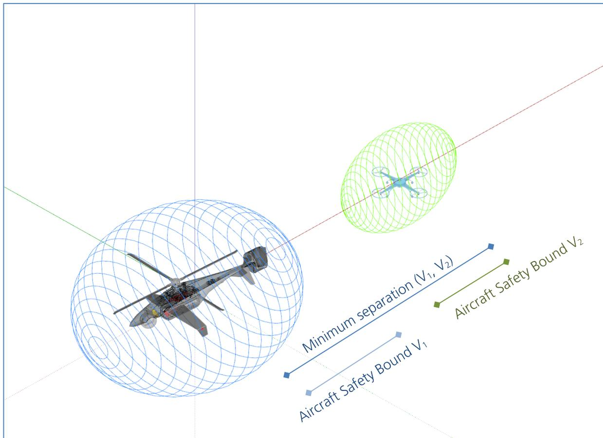
Figure 5: Relative separation distances considering different aircraft types
