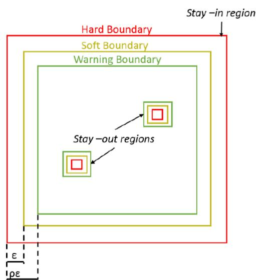
Figure 2: Geofencing Boundaries as introduced by Nasa SAFEGUARD [4]
