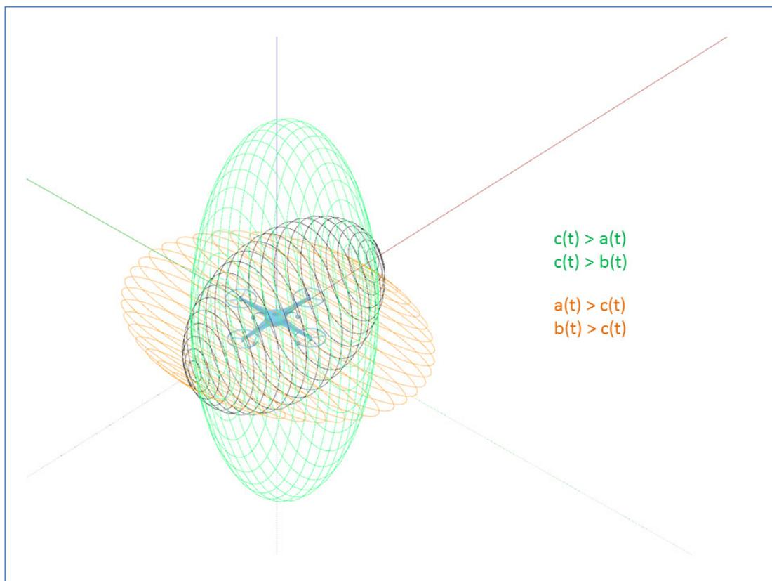
Figure 4: Scaling the Aircraft Safety Bound
