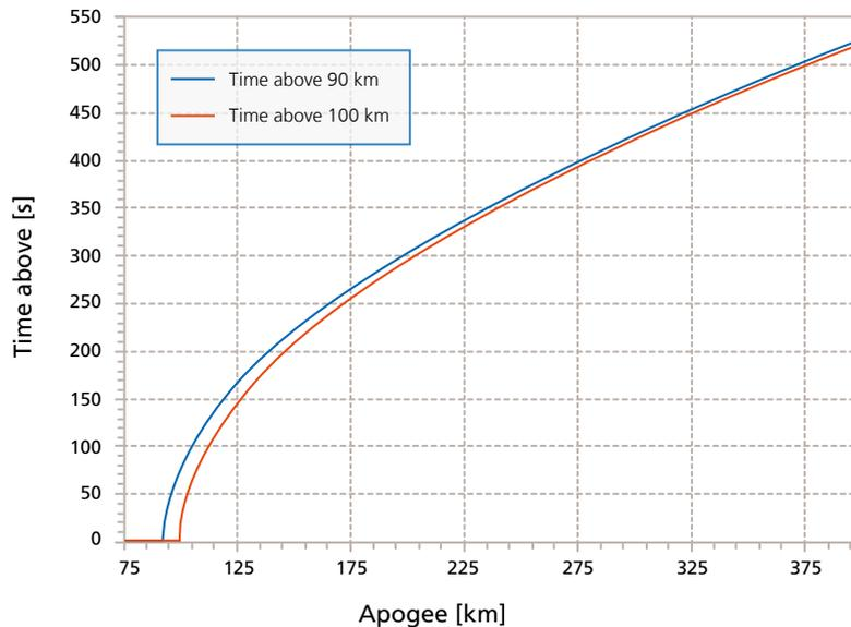
Fig. 5-4 Time spent above 90/100km versus Apogee
