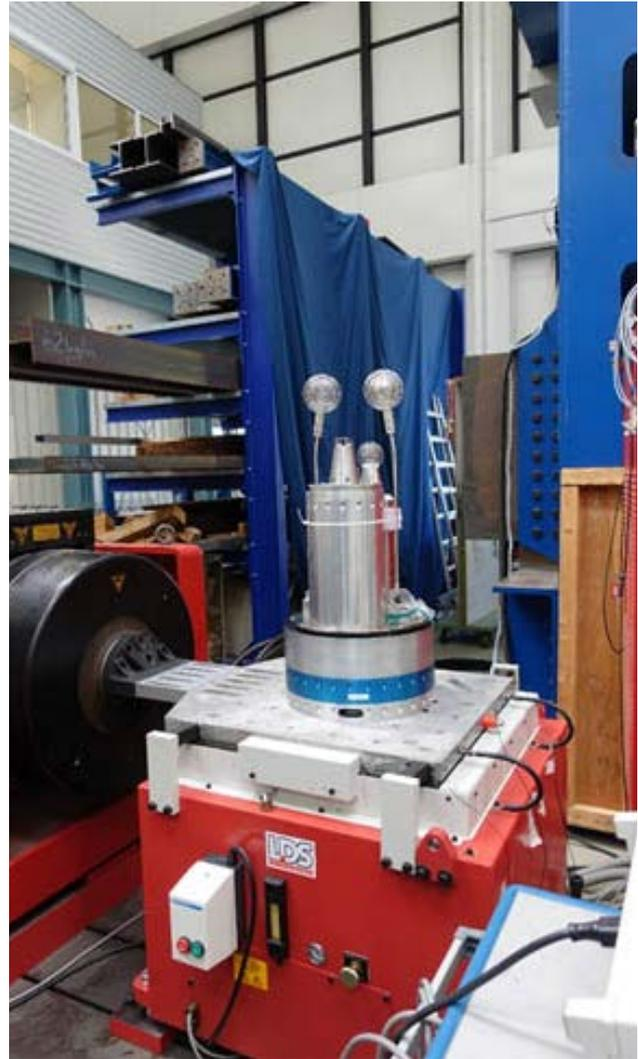
Fig. 7-2 Vibration test run of complete payload (left) and single experiment deck (right)
