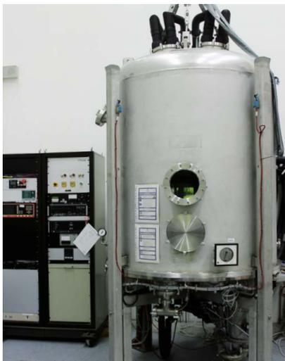
Fig. 7-1 MORABA thermal vacuum chamber
