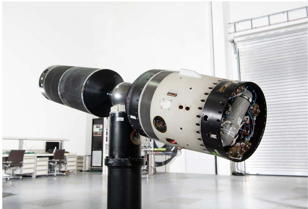
Fig. 7-3 3-D air bearing test for the verification of Cold Gas System control loops
