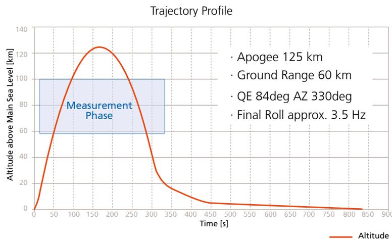
Fig. 3-5 Typical Trajectory of an Atmospheric Physics Mission
