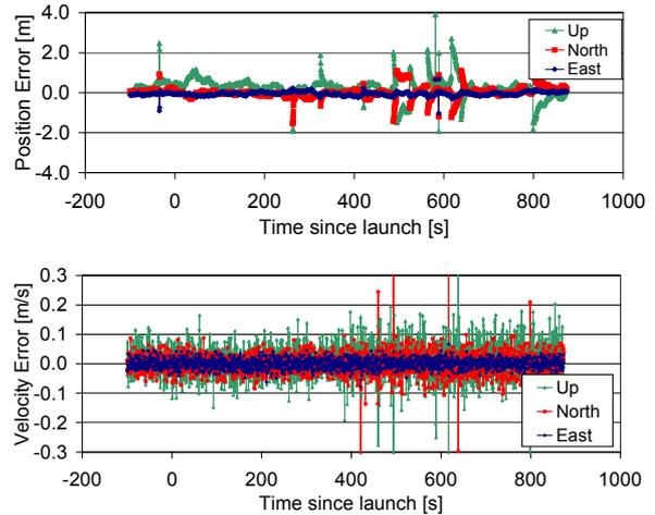
**Fig 6** Position and velocity errors in East, North, and up direction for simulated Maxus scenario in the absence of tropospheric and ionospheric path delays.
