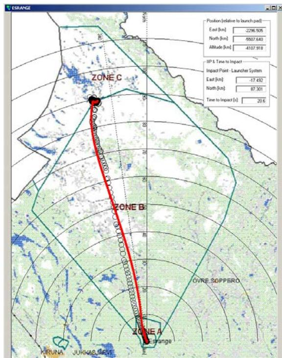
**Fig 9** Plot of Maxus-5 ground track (solid line) and instantaneous impact point predictions (open circles) computed within the Orion-HD receiver.
