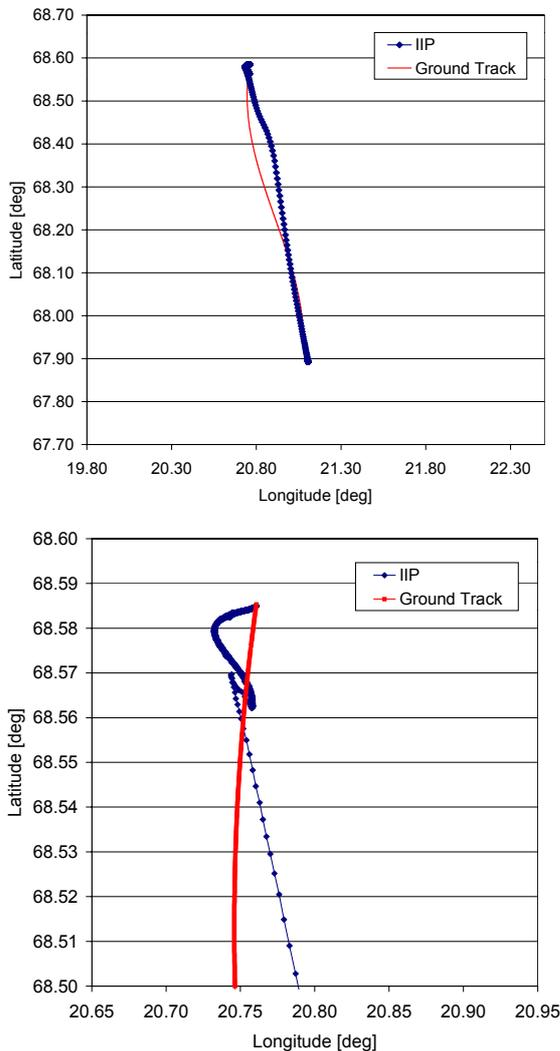
**Fig 7** Onboard IIP results and ground track for simulated Maxus trajectory (*top*: complete flight path; *bottom*: close-up view of landing area).  $0.01^\circ$  in latitude correspond to roughly 1 km.
