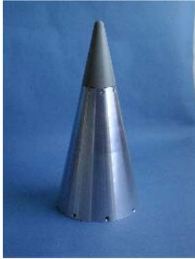
**Fig. 2** Helical tip antenna with radome for GPS tracking of sounding rockets during the early flight phase (DLR Mobile Rocket Base)
