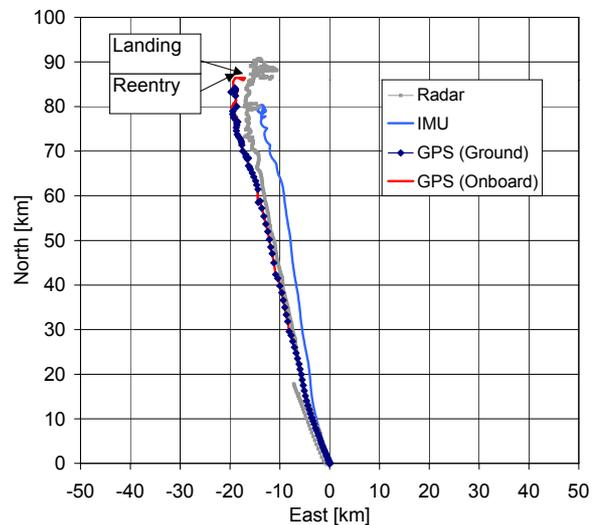
**Fig 10** Comparison of IIP predictions for Maxus-5 using GPS, radar and inertial platform (IMU) data
