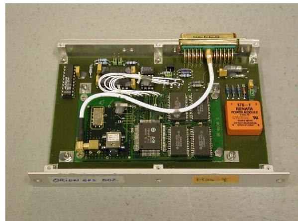
**Fig. 1** Maxus-4 flight unit of the Orion GPS receiver with mission specific interface board (Kayser-Threde)
