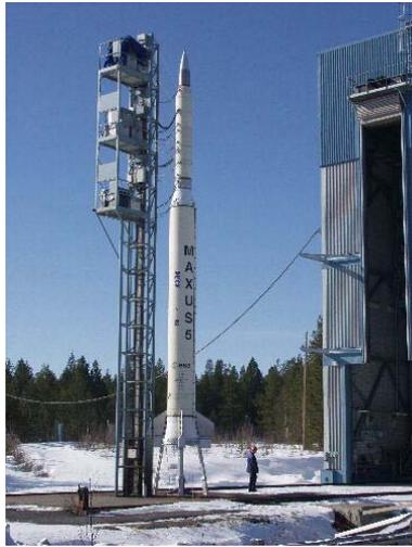
**Fig 4** The Maxus rocket has an overall length of 15.8 m and a total mass of 11.4 tons. It employs a Morton Thiokol Castor 4B motor, which develops a thrust of 430 kN over a 64 s burn time.
