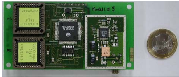
Fig. 3 GPS Orion-HD receiver for sounding rocket tracking and IIP prediction
