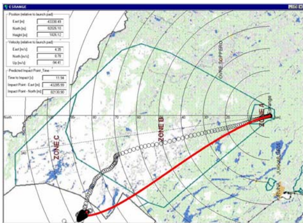
Fig. 4 GPS based IIP predictions (circles) and ground track (solid line) for Maxus-4. North is left and east up on this screen shot of the GPS real-time monitoring system.
