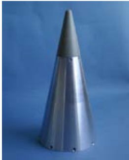
FIG. 3. GPS antenna mounted in the tip of a rocket
