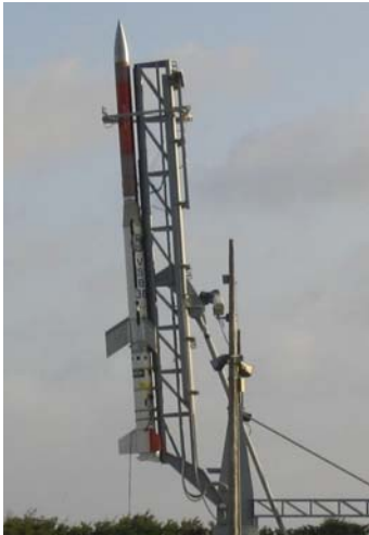
FIG. 10 The VSB30 rocket had an overall length of 12.7 m. It employed a VS31 boost motor and a VS30 second stage motor, which carried a 400 kg payload to an apogee of 240 km
