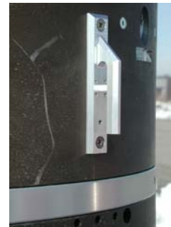
FIG. 4 Blade antenna for GPS applications
