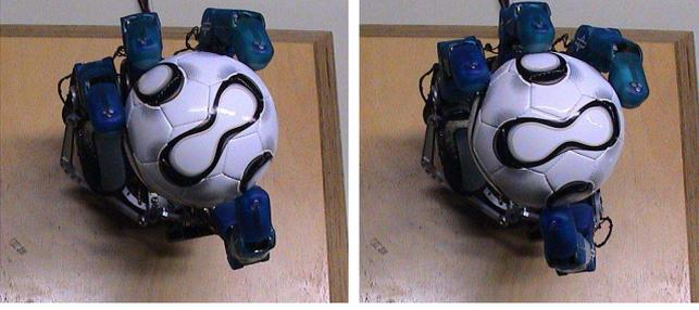
Fig. 4. Hand holding the ball before (left) and after the rotation around the object  $z$ -axis with  $\Delta\beta_{O,z} = 0.6\text{rad}$  (right).
