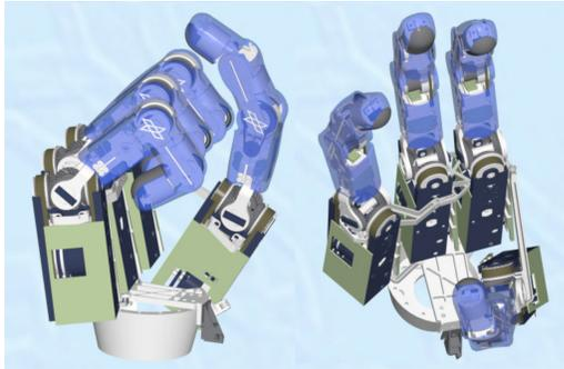
Fig. 2. Power and precision grasp configuration
