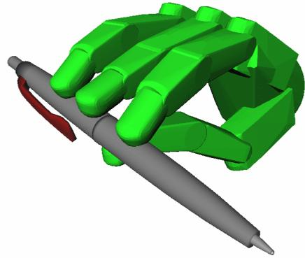
Figure 11: Planned pinch grasp on a pen
