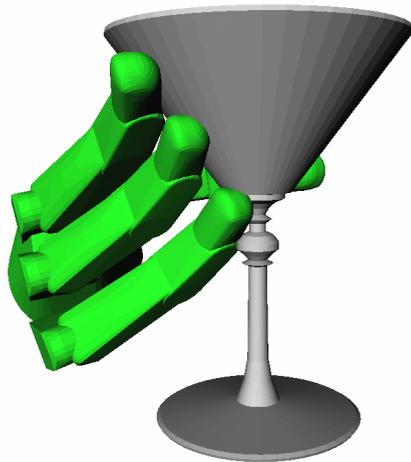
**Figure 12:** Planned pinch grasp on a cocktail glass
