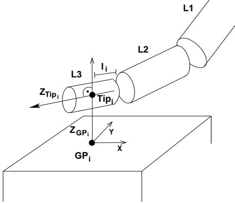
**Figure 6:** Contact situation for a pinch grasp
