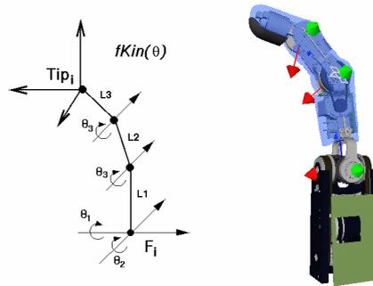
**Figure 4:** DLR Hand II kinematic model of finger.
