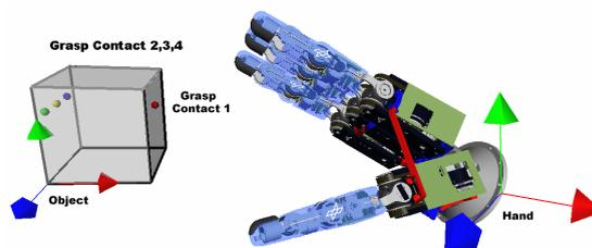
**Figure 2:** How to find a hand configuration (wrist frame, finger joints) for a given grasp contact set?
