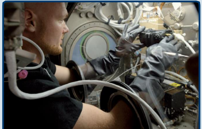
This is the glovebox on the International Space Station, used to perform experiments involving materials or substances that should not be touched or inhaled. Image: NASA/ESA
