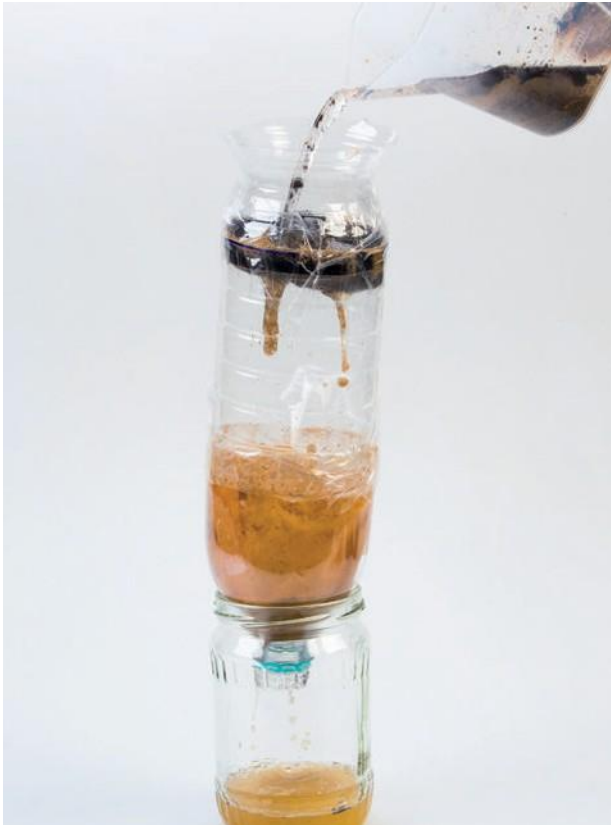
The self-built water treatment plant. Picture: DLR/Timm Bourry
