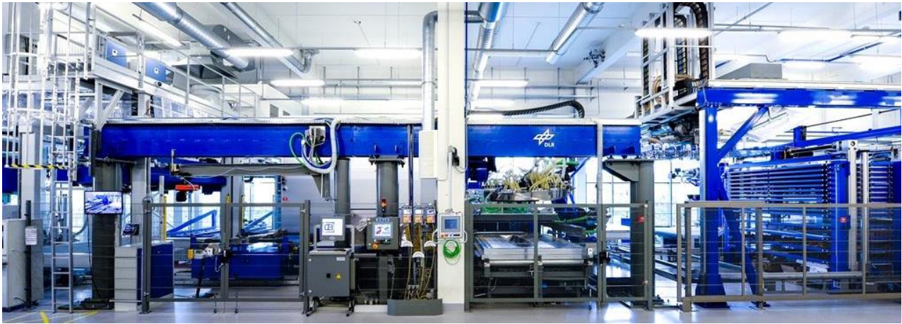
Evo facility – fully automated RTM production line
