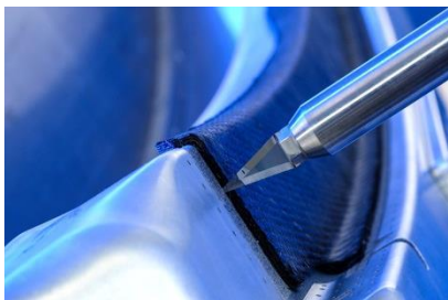
Preform trimming to net-shape geometry by ultrasonic knife
