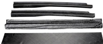
Preform processing: ply, oversized preform, net-shape preform, cured part
