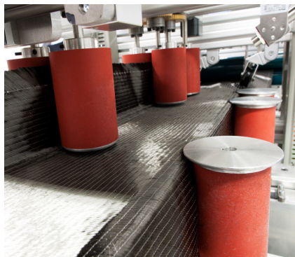
Rollumformung von MAG-Material Roll-forming of NCF-Material
