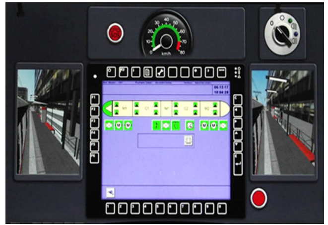
Figure 7-5: Example of rear view display (side part) incoherent with the real direct outside view
