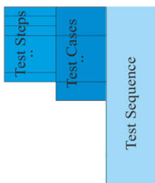
Figure 8-3: Symbolic structure of a test sequence for conformity testing
