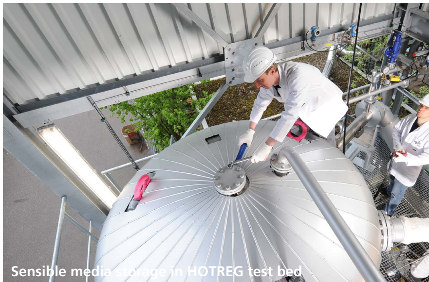
Basalt bulk material for liquid salt in a single-tank storage
