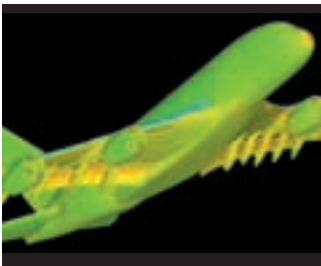
Computational Fluid Dynamics (CFD) on a transport aircraft
