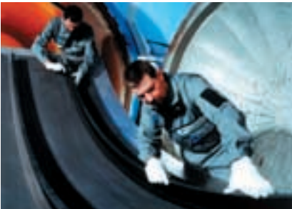
Production of carbon-fibre fuselage sections
