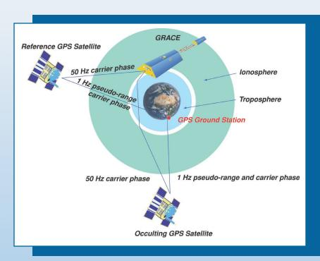
This diagram illustrates how the occultation process works. The GRACE satellite tracks a GPS satellite as it "rises" and "sets" through the limb of the atmosphere, while a second GPS satellite is used as a reference.
