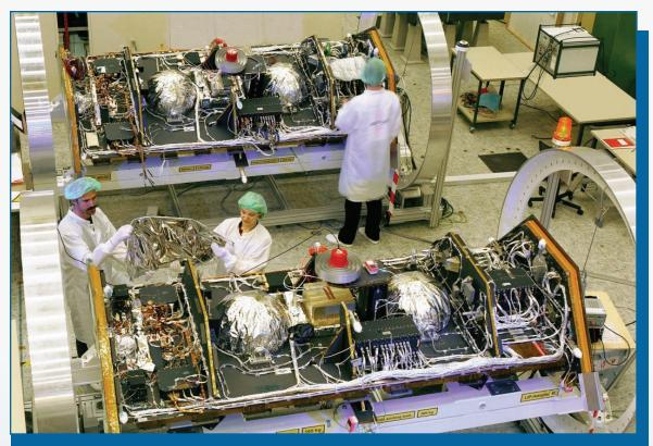
A sneak peak at the innards of a spacecraft! For the GRACE mission, the spacecraft itself is the main instrument. This picture shows the GRACE spacecraft with the solar panels removed and gives a clear view of the various components. It was taken the Astrium test facility in Friedrichshafen, Germany.
