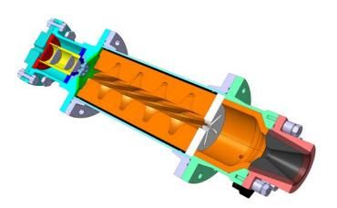
Current status of the AHRES B hybrid rocket engine demonstrator.
