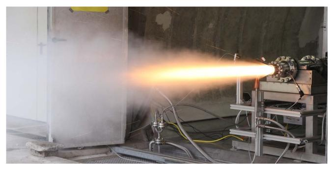
Experimental firing of the AHRES hybrid rocket engine demonstrator at the test bench at DLR Trauen
