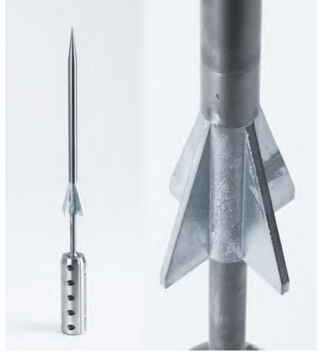
Fig. 1. Photographs of the model: it consists of three separable parts that are screwed together. The fin assembly is cast in gallium, whereas the remaining sections are manufactured from steel.
