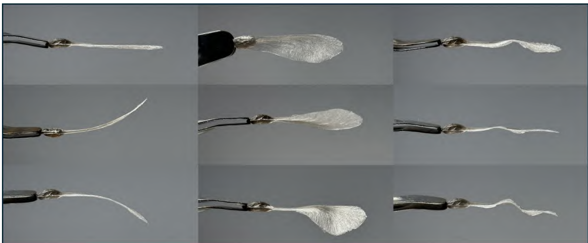
Figure 1: UV resin replica with different curvature profiles produced by thermoplastic reshaping via templates
