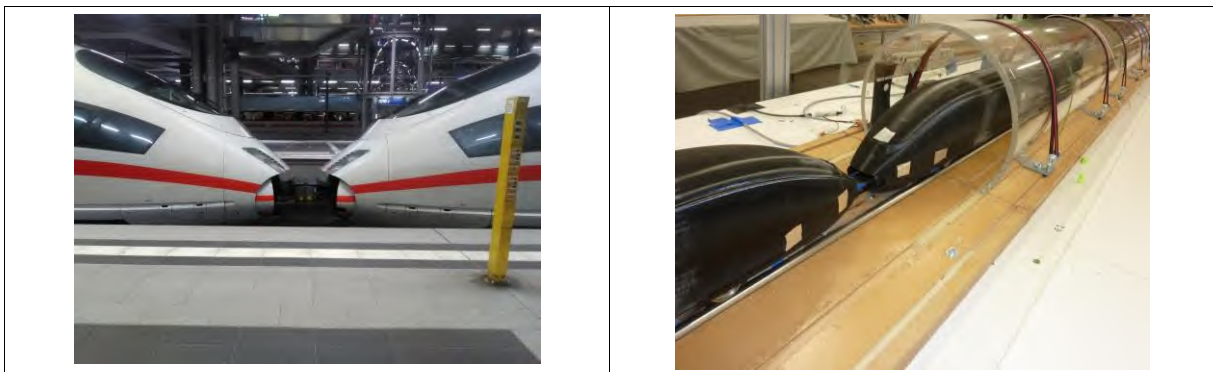
Figure 1: Left: Coupling point of the original ICE3. Right: Model of a coupled ICE3 at the entrance of the model tunnel in the TSG facility.
