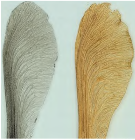
Figure 2: Mikrostructure of the replica (left) vs the original (right)
