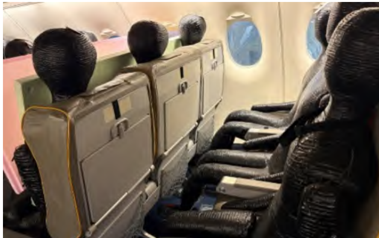
Figure 2. Picture from the measured area of the Donier 728 with a thermal dummie on each seat.
