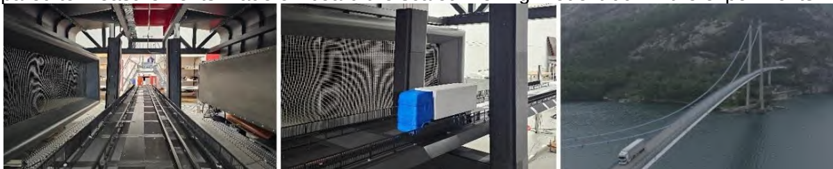
Figure 1: Left : Wind-tunnel setup: 1 :15 model of Lysefjord bridge, towers, railing and (center) generic truck, and (right) the real Lysefjord bridge in Norway.
