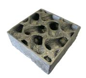
MuSiK: Silicon carbide ceramic gyroide structure (Design by Airbus)
