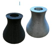
IRAS: Laval nozzle throat Left: 3D-printed green body Right: Converted to silicon carbide ceramic
