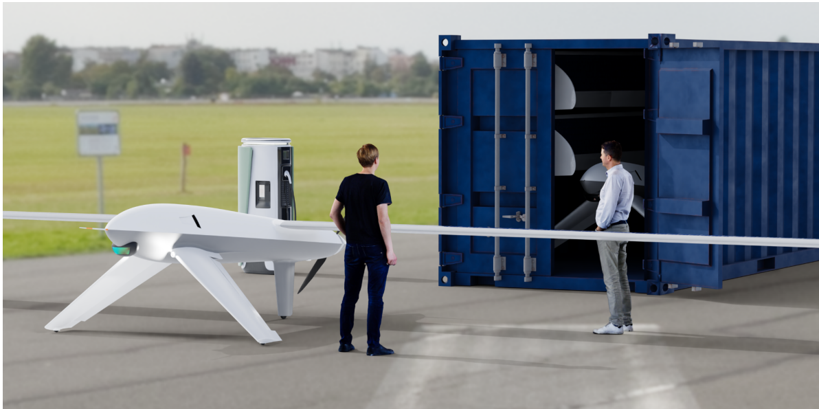
Figure 3.13: Conceptual visualization of HEIKE 's airfield-based charging equipment and transportation container
