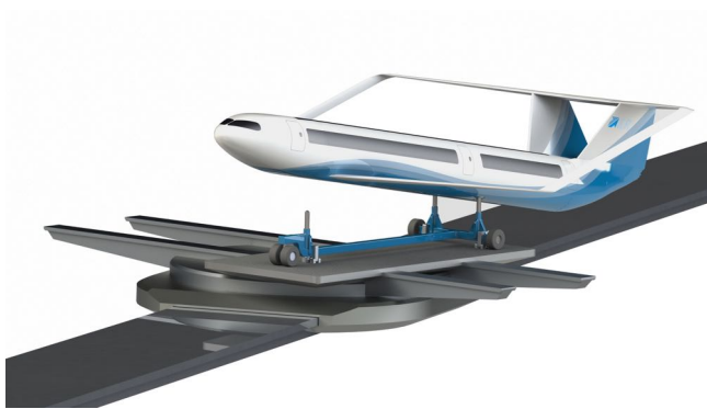
Figure 6.5: Landing with sideslip and lateral displacement
