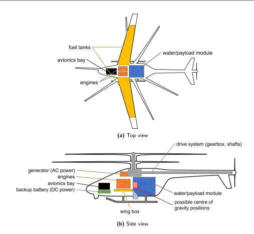
Figure 3.3: Internal component Layout of FireWasp
