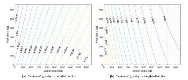
Figure 3.2: Centre of gravity in axial- and height-direction in meter as a function of fuel and water mass
