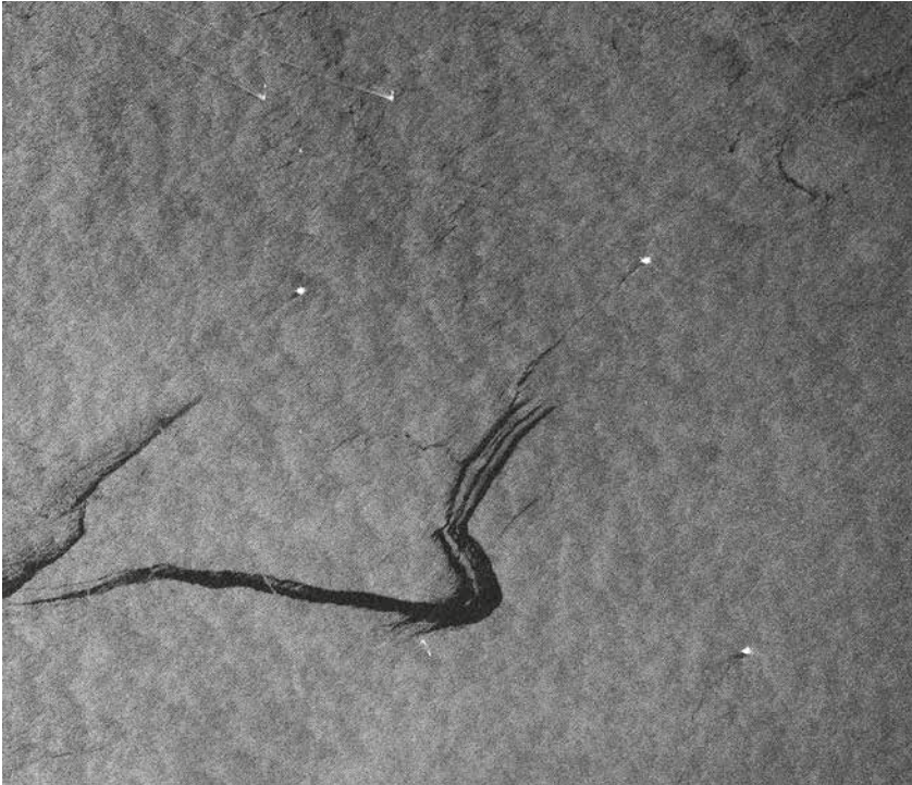
Smooth surfaces such as oil spills or relatively calm water reflect the radar signal away from the satellite, resulting in low backscatter and dark areas in the image. Drilling rigs and ships are visible as bright points on the water's surface.
