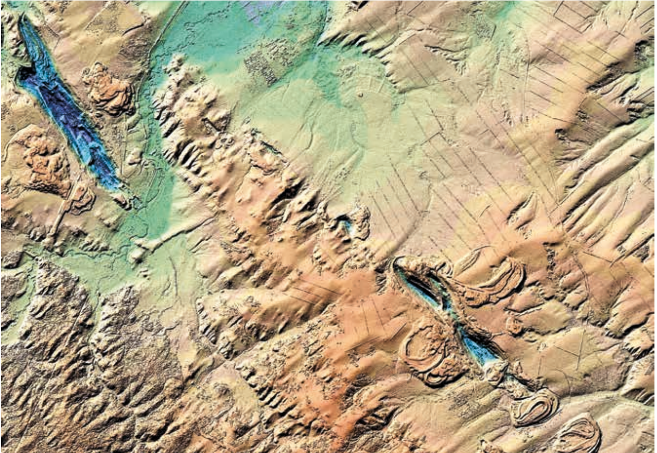
TanDEM-X digital elevation model of open pit mining area in Kiselyovsk, Siberia, Russia (deep pits in bluish colors; the noticeable straight, diagonal lines are forest strips planted to protect the large fields against wind erosion)
