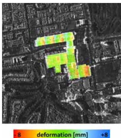
Soon after the launch of TerraSAR-X IMF produced the first spotlight SAR interferograms which revealed surprising details of urban topography and building deformation. The interferometric phase overlaid in color on the image of the Las Vegas Convention Center shows roof deformations due to temperature changes (area: 1.5 km × 1.5 km).
