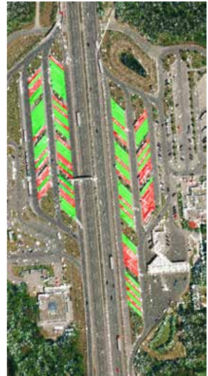
Automatic identification of 64 free (green) and 48 occupied (red) truck parking lots on the rest area Nürnberg-Feucht (A9). Image data: TerraSAR-X, 12.9.2012, 8:26. The aerial image in the background was taken at another time.
