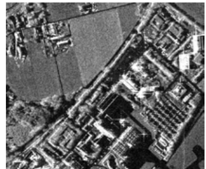
TerraSAR-X high resolution spotlight image of DLR Oberpfaffenhofen with a resolution of approximately 1 m (top). The new staring spotlight mode provides up to 25 cm azimuth resolution or an improved radiometry as shown in this image (bottom).
