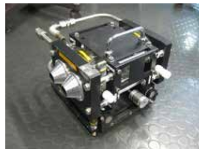
IMF-developed absorption cell for the Bruker IFS 125HR sample compartment with an absorption path of 22 cm, applicable to a temperature range 190 – 350 K. The cell body is a double-jacketed glass tube. The windows are mounted on stainless steel flanges coated with PFA. The window openings with baffles can be seen.
