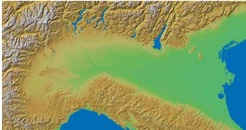
Digital surface model (DSM) of northern Italy generated from more than 400 Cartosat-1 scenes after bundle block adjustment
