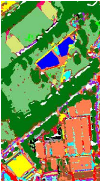
Factor graph based information fusion classification of WorldView-2, TerraSAR-X and Digital Surface Model data for 23 classes for a part of Munich city. Specific classes are e.g. glasshouse, different grass species and tennis courts.
