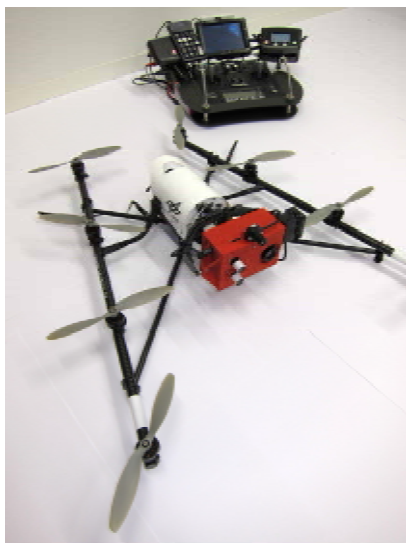
IMF's Flying Wildlife Finder, based on a Falcon 8 octocopter
