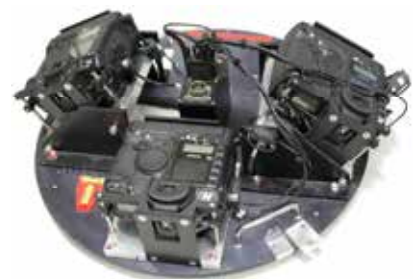
3K camera system consisting of 3 off-the-shelf Canon cameras mounted on a ZEISS frame, for acquiring sequential images at a frame rate of up to 5 Hz
