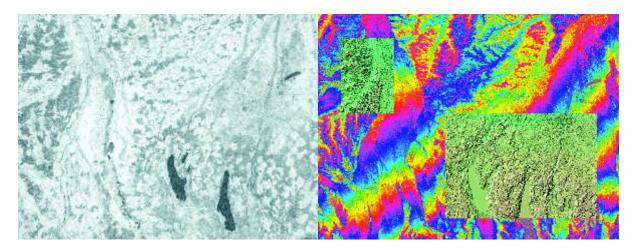
Coherence map at left and interferogram at right, the latter superimposed with two segments of a digital elevation model.
