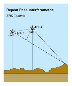
The two images can be recorded either at the same time using one transmitreceive antenna and a second receiver antenna placed some distance away (lower figure), or with a time lag by recording a second image during a second flight over the relevant area from a slightly different orbit (figure at left). The first case is called **singlepass interferometry**, the second **repeat-pass interferometry**.
