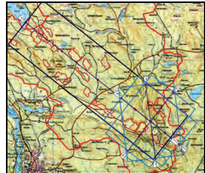
Figure 3-24: BIOSAR 2008 mission planning – Flight strips over a part of the Krycklan forest area, Sweden. Multi-baseline flights in L- and P-band (dark blue) and a smaller part of the test site additionally observed in viewing angles of 45 and 90 degrees (light blue) with L- and P-band for polarimetry.
