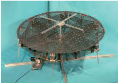
Figure 2-42: Bread-board of the MAPSAR antenna main reflector.
