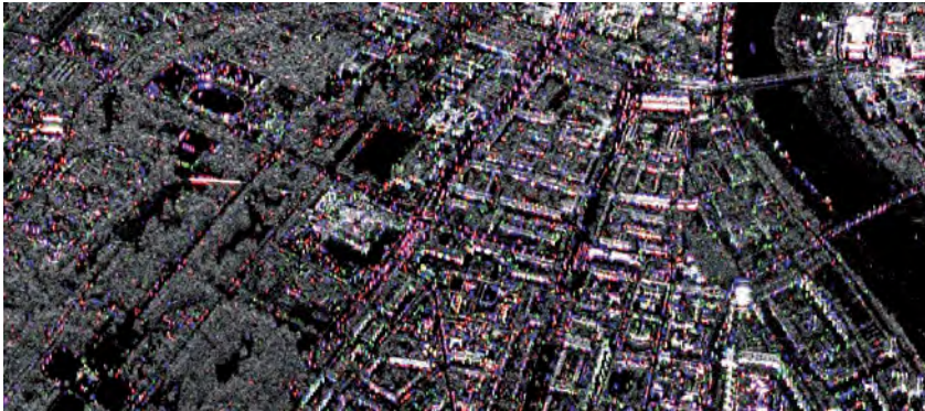
Figure 3-36: Coherent scatterers in the historical city centre of Dresden, Germany, at different polarisations: HH (red), VV (blue), HV (green), right: river Elbe.
