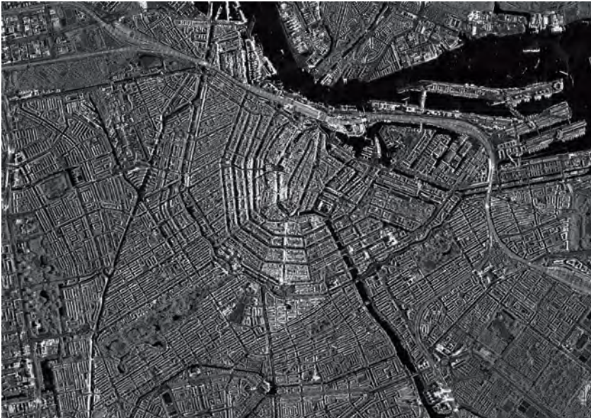
Figure 2-10: This 150 MHz TerraSAR-X Spotlight image of Amsterdam and its many canals was taken on December 9, 2008.
