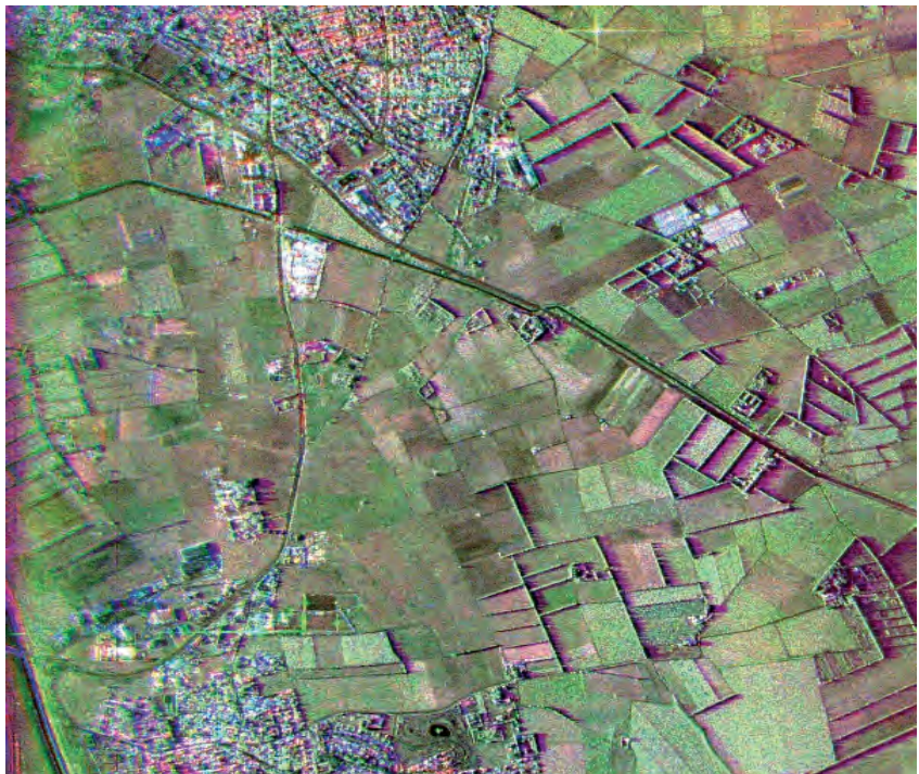
Figure 4-10: Colour composite of three SAR images with different bistatic angles, showing the clear differentiation of surface features.
