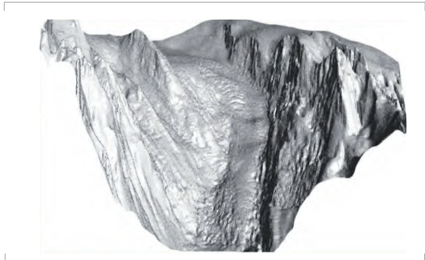
Figure 3-12: OMEGA: Digital Elevation Model of Engabreen – the glacier tongue of Svartisen, Norway acquired at X-band using single-pass SAR interferometry. The height varies by approx. 1500 meters in this sub-image of ca. 2 km x 2 km.
