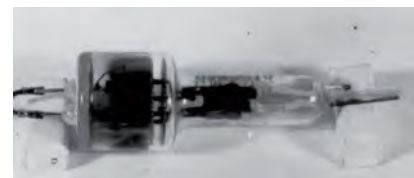
Figure 1-22: A (probably) two-slit magnetron valve for cm-wavelengths from DVG valve laboratory.
