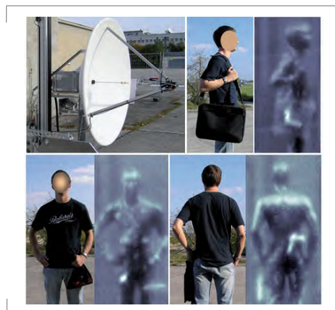
Figure 4-98: Photograph of the LPAS-2 radiometer imager (upper left), and corresponding photographs and 90 GHz imaging results of a person carrying various optically non-visible objects.
