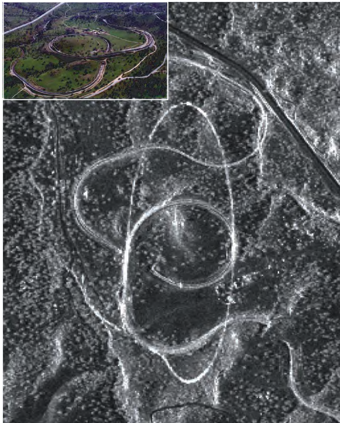
Figure 2-16: Trainspotting with TerraSAR-X: This image shows a valley located approx. 100 km north of Los Angeles, California. It contains the highway 58 (dark line) and a railway (bright line) connecting Bakersfield to Mojave, crossing the Tehachapi Pass. The Tahachapi Loop was built to reduce the slope and can be recognised as the bright circle in the center of the image. The bright circle is the railway track; the ellipse touching the circle is a very long, running train which appears displaced from the tracks. The displacement between the train and the rails in azimuth direction is a SAR effect for objects moving in range direction. For this imaging geometry, the speed of the train can be estimated from the azimuth displacement of 360m to 25 km/h.
