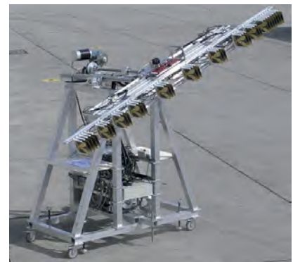
Figure 4-100: Photograph of the ANSAS multi-spectral hybrid radiometer system combining aperture synthesis and mechanical scanning for two-dimensional imaging. More than 15 antennas are used in order to provide similar electromagnetic properties for those antennas connected to the 15 receivers.
