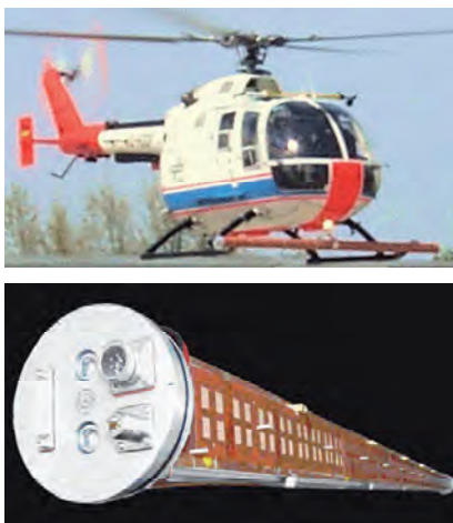
Figure 4-12: Top: Antenna system attached to the skids of the helicopter. Bottom: SIREV antenna with 56 receiving subarrays.
