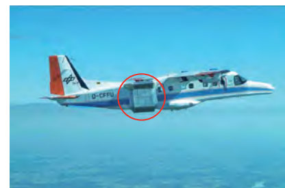
Figure 3-45: F-SAR antenna mount (red circle) under test. The aerodynamic properties are being investigated. The new antenna mount allows an easy exchange of individual antennas in the future.
