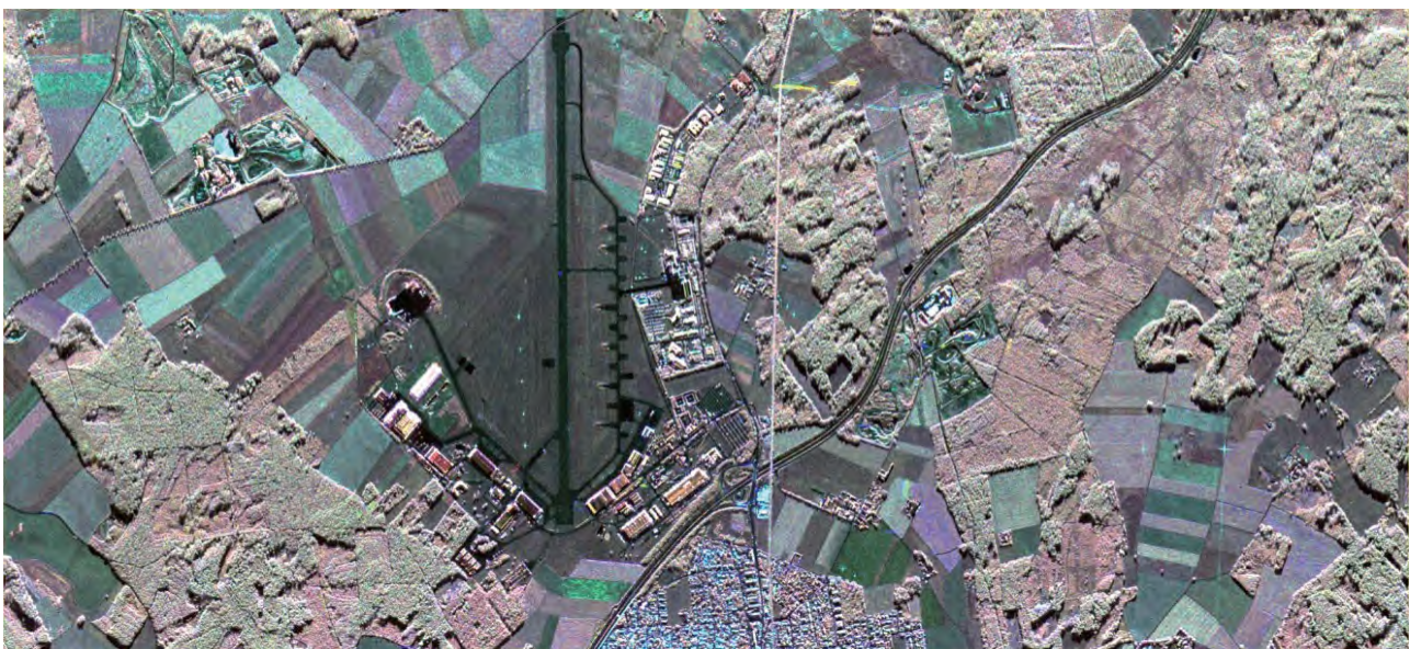
Figure 3-5: Fully polarimetric E-SAR image of Oberpfaffenhofen, incl. DLR facilities in image centre; composite obtained from two dual-polarized data takes in C-band (HH-green, HV-red, VV-blue), corner reflectors (light blue) aligned with the runway.
