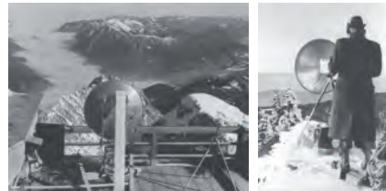
Communication experiment: 5 cm transmitter on the Zugspitze (left photo), receiver on the 250 km distant Mount Arber, 1939.
