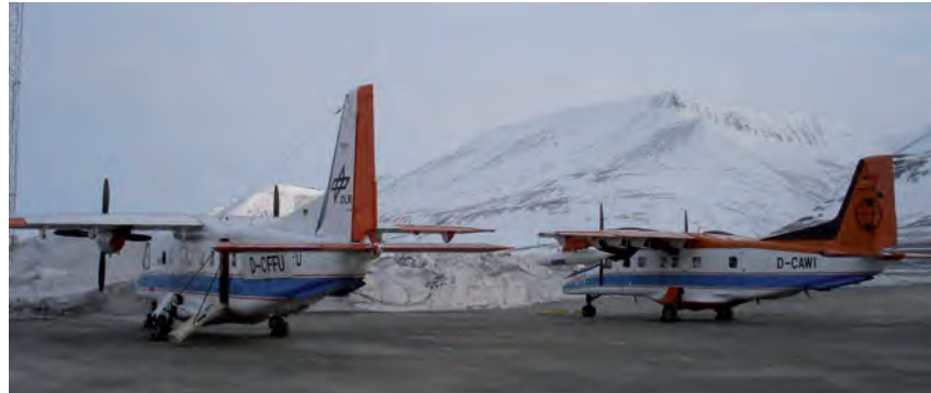
Figure 3-17: SVALEX 2005 – The two Do228 research aircrafts D-CFFU of DLR (left) and D-CAWI of AWI (right) at Longyearbyen airport in Svalbard. Instruments flown: E-SAR on D-CFFU and the Meteo-Pod, laser altimeter, line scan camera and surface temperature instrument on D-CAWI.
