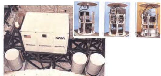
NAVEX on Spacelab, D1 mission: Antennas T/R (left) and receiver, atomic clocks (Cs/Rb) and receiver (right).
