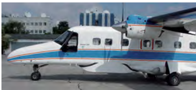
Figure 4-74: P-band antenna with the wind deflector mounted under the fuselage of DLR's Dornier Do 228.
