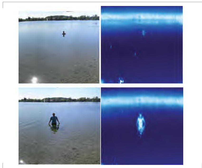
Figure 4-95: ABOSCA imaging result of a person approaching the beach of a lake from the waterside. The distance was about 15 m and 8 m.
