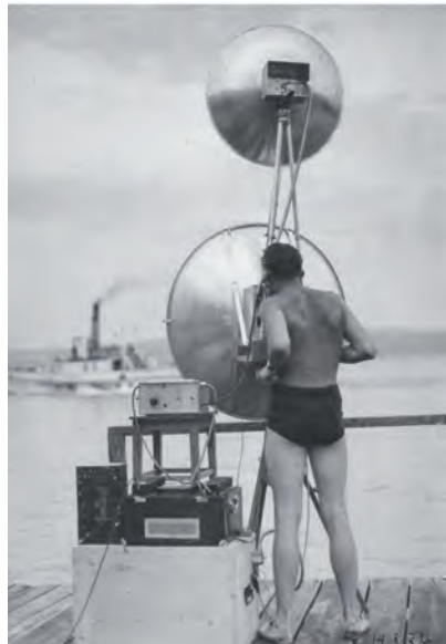
Figure 1-19: The first CW radar of the DVG during experiments in 1937 at Lake Ammersee.
