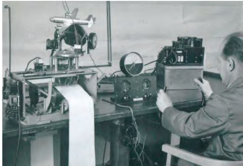
Figure 1-31: Experimental assembly of an analogue computer for an automatic landing process at Riem, about 1955.
