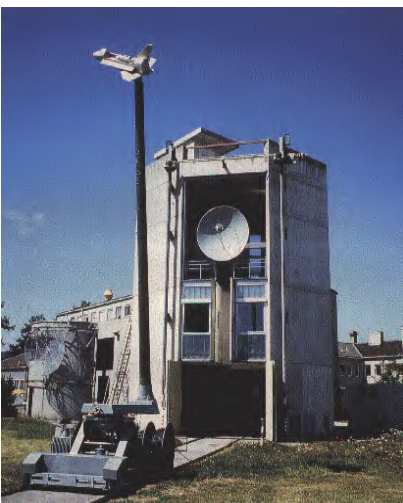
Figure 1-39: The AMA antenna test range measuring a scaled down Space Shuttle.
