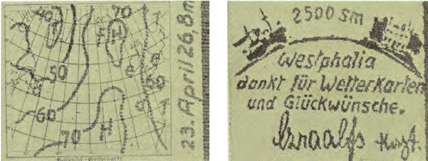
Figure 1-6: Radio weather map sent in 1926 from Radio Norddeich to the "Westphalia" over 4600 km via the DVG radio technique with a thank-you and congratulations message from the ship's captain.
