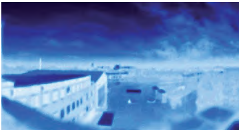
Figure 4-93: Panoramic photograph of a typical scene for surveillance applications and the corresponding 90 GHz radiometric image.
