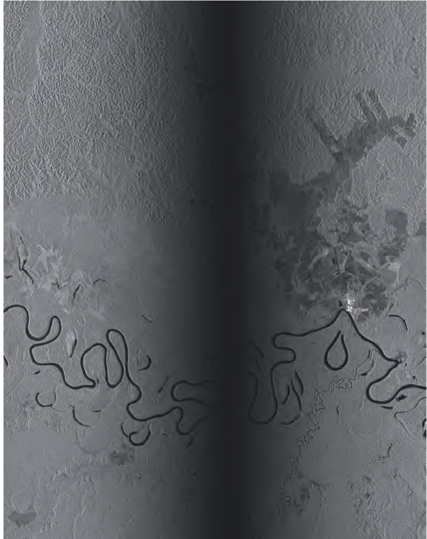
Figure 2-12: Image over the Amazon rain forest acquired with a notch beam pattern. The gamma profiles derived from such images show a well established drop around the position of the pattern null. Using fitting techniques this position and hence the antenna beam pointing can be determined with milli-degree accuracy.
