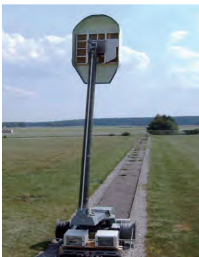
Figure 4-80: DLR's airborne P-band SAR antenna mounted with its wind deflector on the antenna measurement facility AMA.
