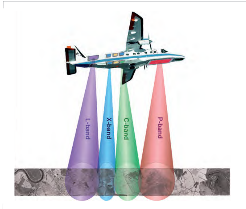
Figure 3-43: An Artist's view of F-SAR acquiring data simultaneously in X, C, L and P-band.
