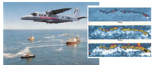
Multi-frequency radiometer MERES, oil spill imaged in 89, 36 and 18 GHz (right, top down).
