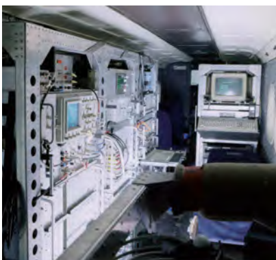
Figure 1-45: View inside the cabin of the DO228 aircraft. The racks are approximately 1.2 m high.
