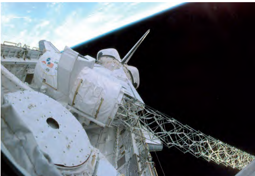
Figure 2-1: View into Endeavour's cargo bay with the deployed 60 m SRTM mast (By courtesy of NASA).
