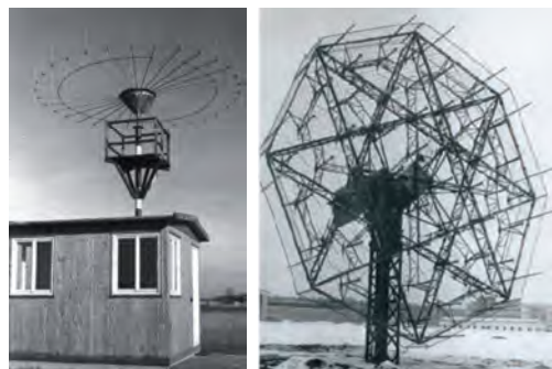
Experimental set-up of an electronic switched direction finder (left), VHF monopulse tracking antenna for satellite signal reception, diameter 11 m (right).
