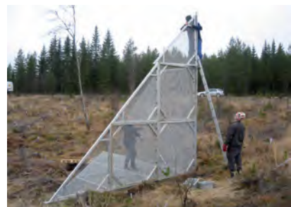
Figure 3-25: Boreal forest at the Krycklan test site in mid Sweden (above) and a meshed corner reflector with side length of 5 m deployed at the test site (below).
