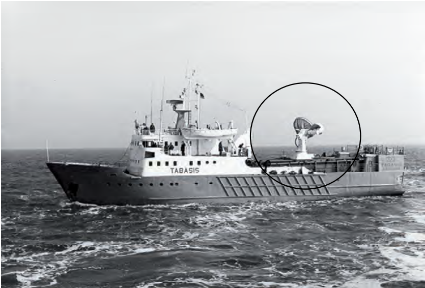
Figure 1-38: The experimental ship terminal (ringed) on its way to the Faroe islands. The antennas were mounted on a container housing the electronic equipment (hidden in the cargo bay).
