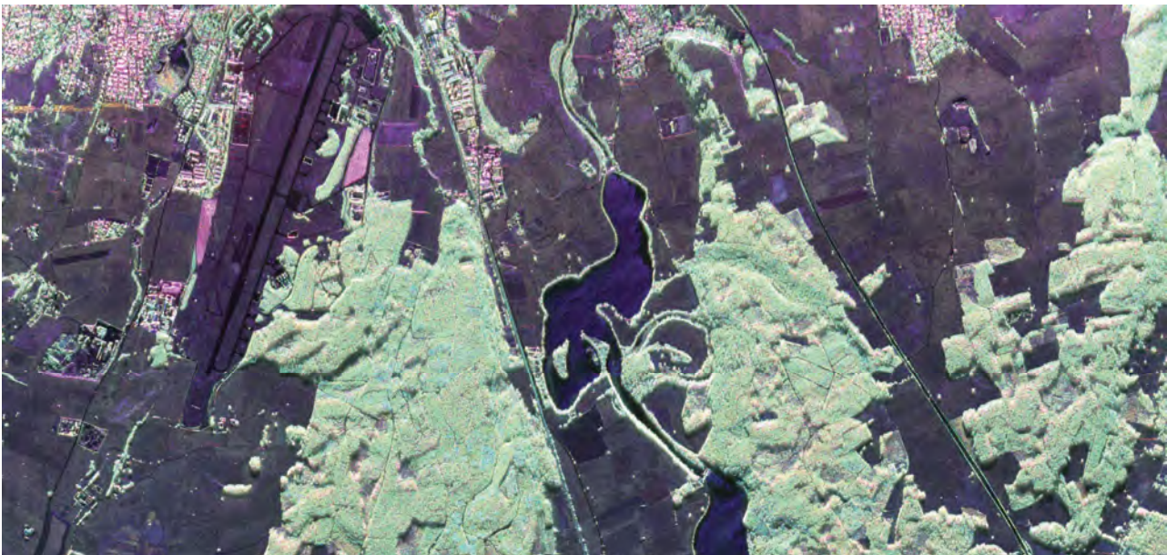
Figure 3-4: The new DLR airborne SAR calibration site at Kaufbeuren, Germany: A former military airfield. Corner reflectors (purple) aligned with the runway. Radar Geometry Image Product (RGI) example: E-SAR L-band, fully polarimetric, high resolution. HH (red), HV (green), VV (blue). Image size: 3 km ground range, 7.5 km azimuth.
