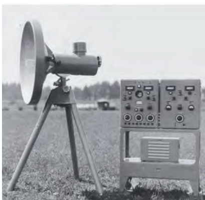
Figure 1-24: Magnetron transmitter of the DVG for RCS measurements of 1:10 scaled aircraft models. This microwave source delivered 10 W CW power at \lambda = 5.2 cm.
