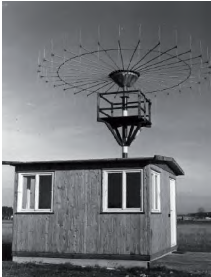
Figure 1-33: Experimental installation of an electronically switched Doppler direction finder.
