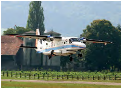
Figure 1-44: The E-SAR of DLR, operated by the Institute, P-band antenna underneath the cockpit.
