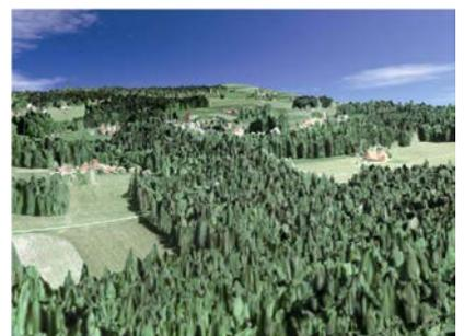
Tandem-L: Simulation of the forest height derived from two radar acquisitions using polarimetric SAR interferometry. The forest biomass can be estimated from the forest height using an allometric equation and the forest profile. This image shows the area of Traunstein, Germany.
