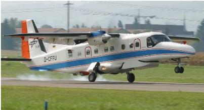
F-SAR: The new airborne SAR system of DLR.
