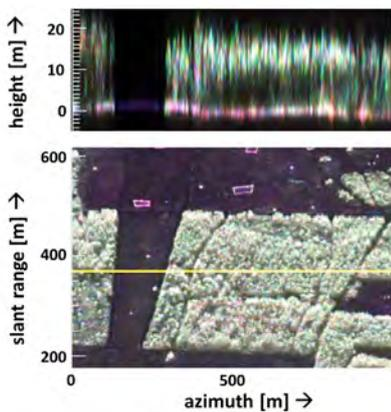
Demonstration of tomographic imaging of a group of trees in L-band. In this example, the radar data were recorded using DLR's airborne SAR system by making several passes at intervals of a few minutes.
