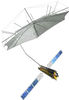
Tandem-L satellite with reflector antenna
