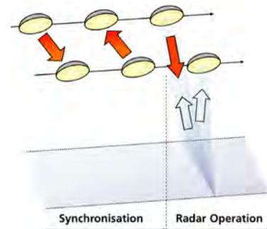
To synchronise the radar systems, short pulses are exchanged between the satellites. This permits a synchronisation at picosecond accuracies.
