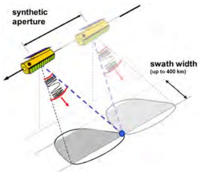
Synthetic aperture radar (SAR). The formation of a synthetic aperture several kilometers long enables a high-resolution independent of the range distance.
