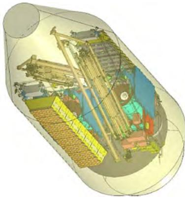
Two Tandem-L satellites in the fairing of a Falcon 9 aircraft
