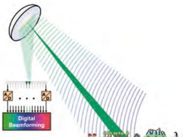
Use of innovative technology on Tandem-L. The digital beamforming technology for high resolution radar systems was developed and patented in a close collaboration between DLR and German industry.
