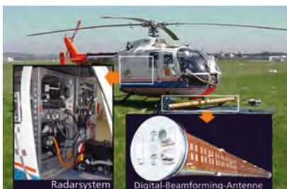
Digital beamforming demonstrator on a DLR helicopter
