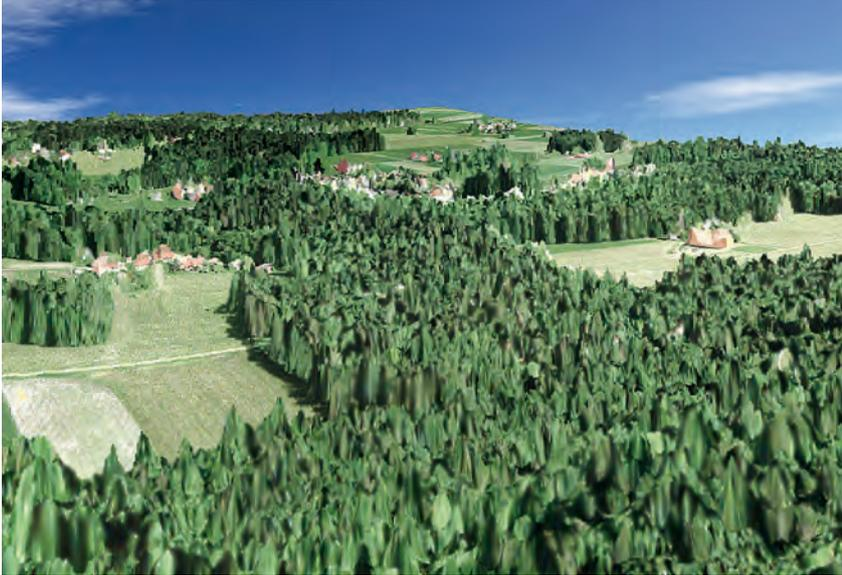
3D representation of the Stadtwald forest in Traunstein, Germany. The forest height was derived from radar data using polarimetric SAR interferometry.
