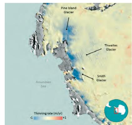
Between 2011 and 2013, the western antarctic ice shield lost more than 150 cubic km of ice yearly. The figure shows changes in the ice height measured by the ESA altimeter CryoSat. Tandem-L will permit continuous monitoring of the ice shield with high spatial and temporal resolution.
