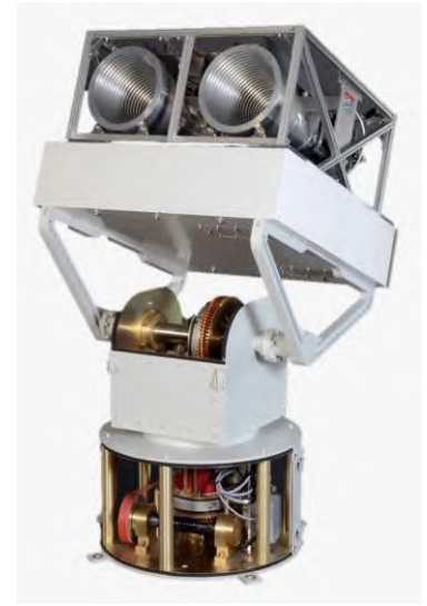
Figure 2.2-39 “Kalibri” C-band transponder developed for Sentinel-1
