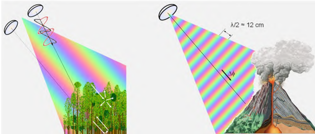
Figure 2.1-27 The two basic measurement modes of Tandem-L. Left: The 3-D structure mode employs polarimetric SAR interferometry and coherence tomography to measure tree heights and vertical vegetation profiles. The individual contributions from ground and canopy can be separated via their polarimetric signatures, and the corresponding heights can be measured by across-track interferometry and multi-baseline tomography. Right: The deformation mode employs repeat-pass interferometry to measure surface deformations with millimetric accuracy.
