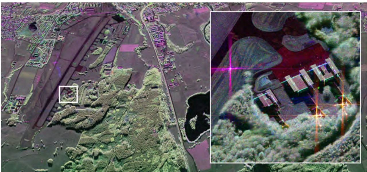
Figure 2.3-11 First fully calibrated DBFSAR image acquired over the F-SAR/DBFSAR calibration test site in Kaufbeuren (HH=blue, VV=red, HV=green). The inset zoom into a small part of the scene illustrates the high-resolution capabilities of DBFSAR.
