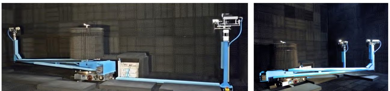
Figure 1.3-5 Microwave anechoic chamber for the measurement of monostatic and bistatic radar signatures
