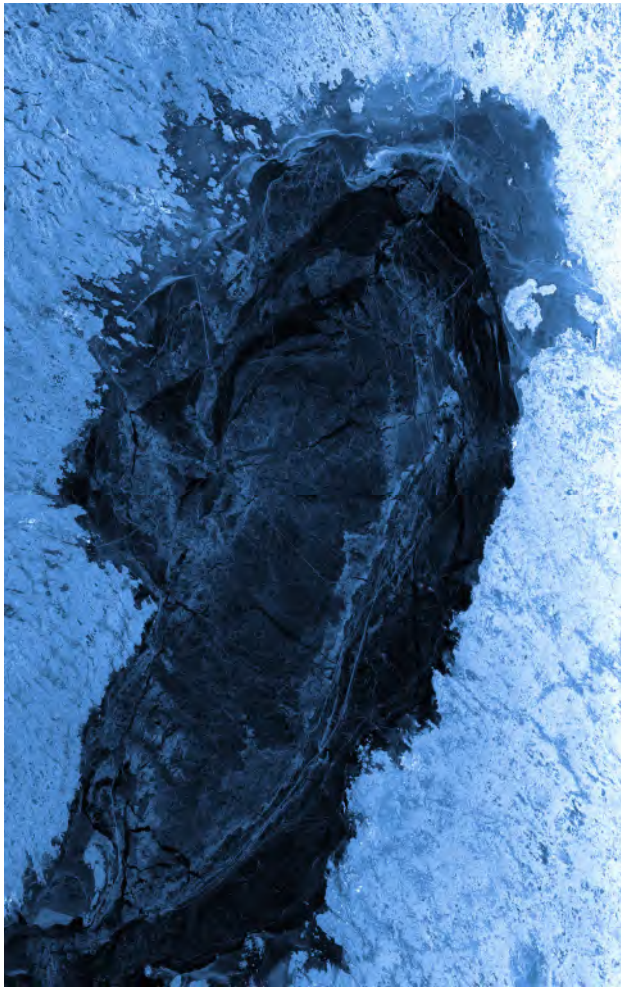
Figure 2.1-4 Wide ScanSAR image of the Gulf of Bothnia acquired on March 6, 2018. At a resolution of \sim 40 m the image extends over 315 km in azimuth at a swath width of 240 km and is composed of six subswaths. The sea is still frozen and the linear tracks are most likely from ice breakers.
