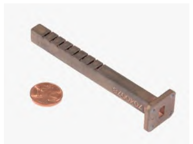
Figure 2.2-81 Ka-band slotted waveguide antenna prototype out of 3-D printed plastic metalized with copper
