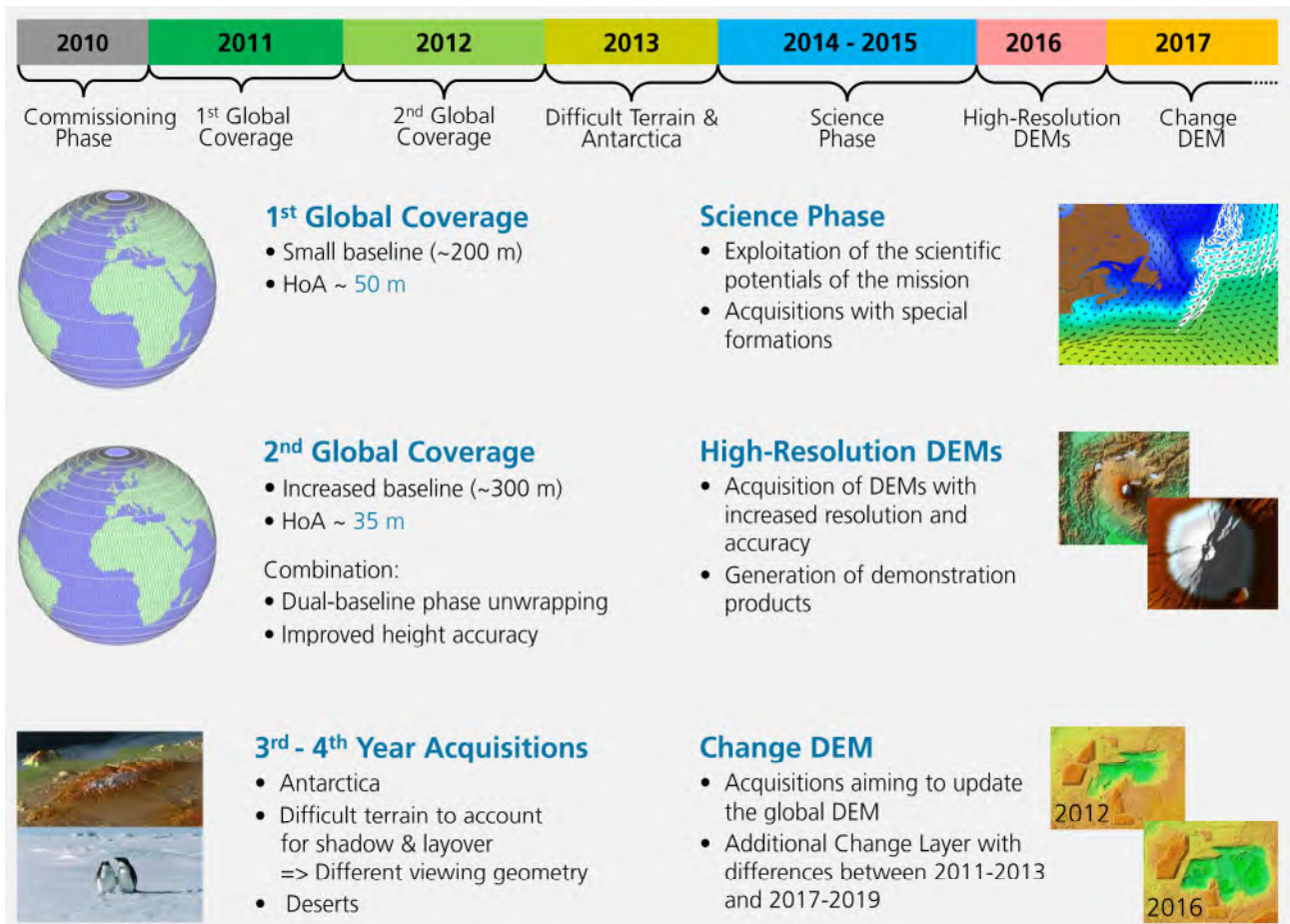
Figure 2.1-10 Mission phases of the TanDEM-X mission. The acquisition of data for the global Change DEM started in 2017 and will last until beginning 2020.
