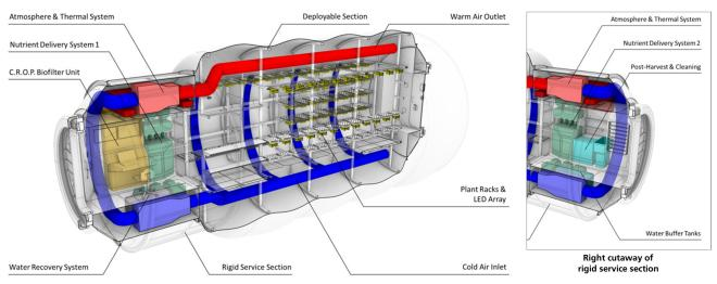
Figure 3: Left and right cutaway of the DLR BLSS test demonstrator.
