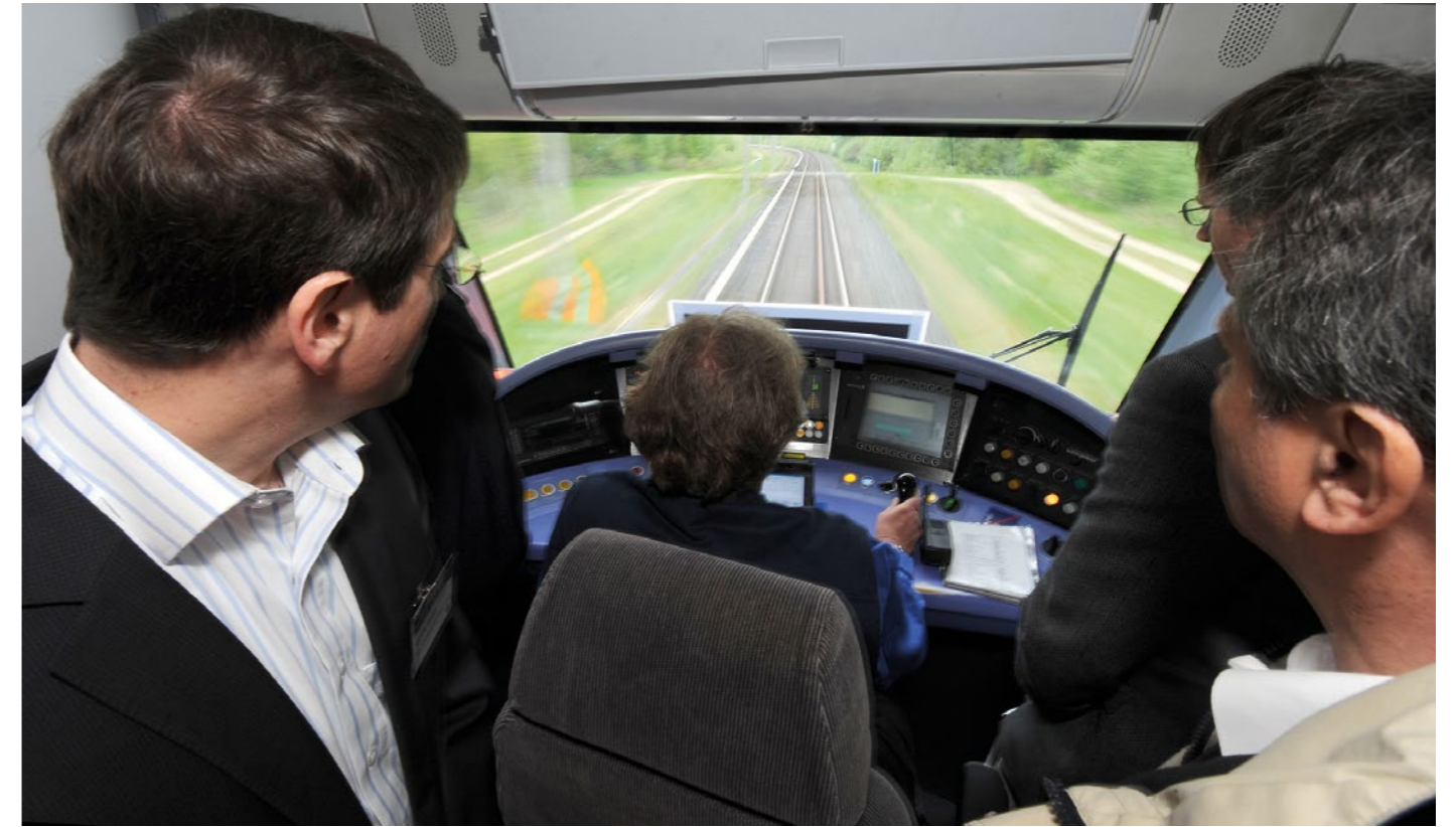
First journey with an anti-collision system for trains. The public demonstration of the Railway Collision Avoidance System, RCAS, conducted in a real train on a test track at the Bayerische Oberlandbahn in 2010 was successful. Since then, the system, which was designed at DLR, has been implemented by industry.
