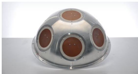
Individual antenna elements combined in an array make navigation more reliable
