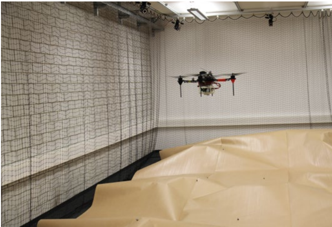
This autonomous multicopter is part of a swarm. Each swarm member autonomously maps its surroundings using ultrasonic sensors. During testing, ground profiles are simulated with a tarpaulin. The individual measurements are communicated to other swarm members so that an overall picture of the environment is created.
