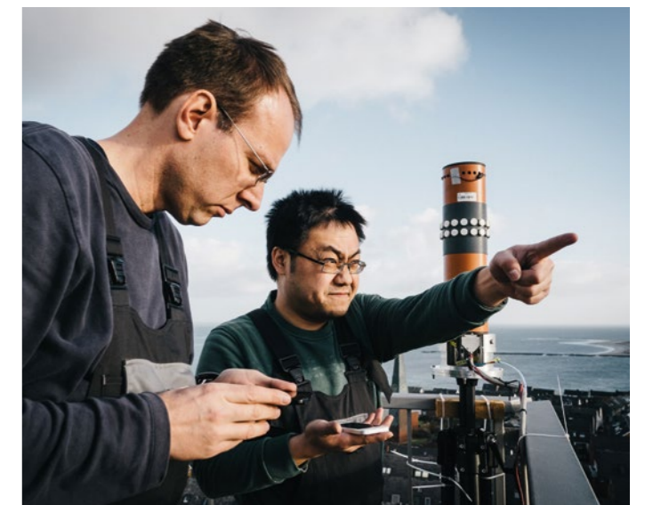
The orientation and position of the antenna must be accurately determined so that the data acquired can be analysed in the home laboratory
