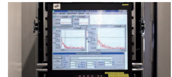
The Channel Sounder consists of a transmitter and a receiver unit. The receiver reveals how the radio signal is reflected by the environment.
