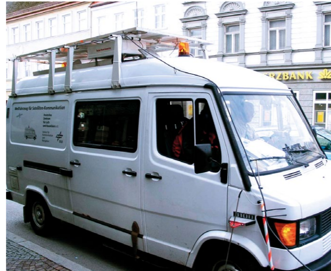
In the first satellite Channel Sounder campaign, the receiving unit moved through Munich city centre in a measurement bus.
