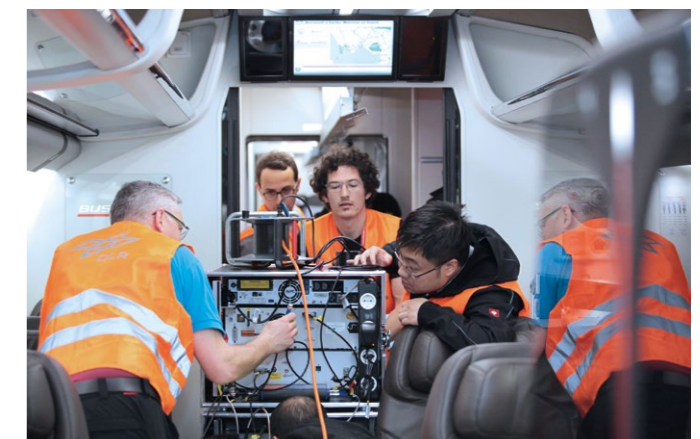
In two moving high-speed trains, DLR experts investigated the propagation of radio waves for train-to-train communication in Italy.
