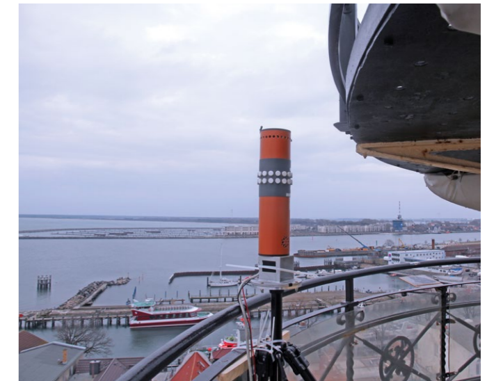
During a measurement campaign in 2014, during which the researchers examined the radio link between a ship and the mainland, the receiving antenna was installed on the Warnemünde lighthouse. In 2016, one team recorded the transmission channel between two ships (DLRmagazine 148/149 reported about this).
