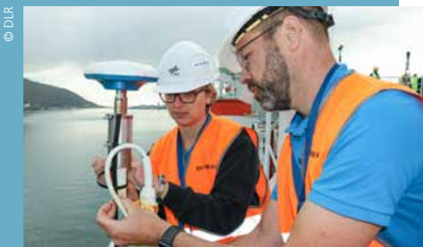
Simon Plass and satellite navigation expert in the DLR MOSAiC team, Friederike Fohlmeister, mount the receiving antenna on the sounding deck. They were responsible for water- and cold-proofing the installation.
