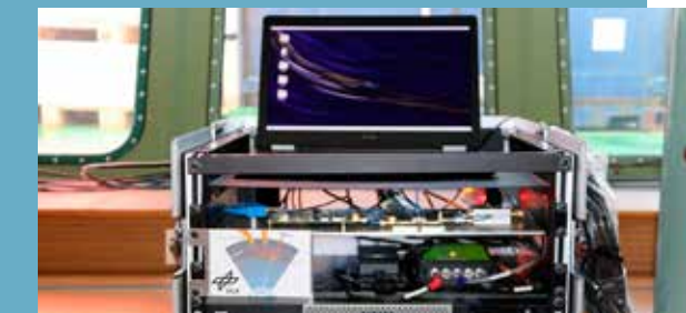
DLR's scintillation recorder – the heart of the measuring on board the Polarstern.
