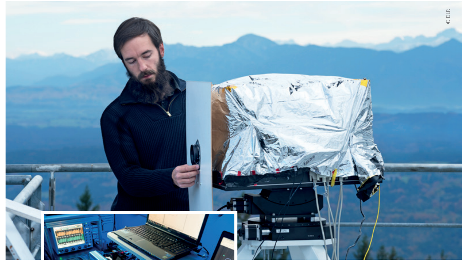
Satellite terminal emulator at Hohenpeißenberg, Upper Bavaria, near Weilheim. DLR scientist Juraj Poliak prepares the testbed for the next communications experiment.
