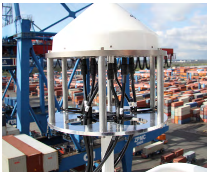
Measurements made on board a container ship have revealed that satellite signals are particularly distorted at ports. This antenna can target an eliminate the effects of jamming transmitters.
