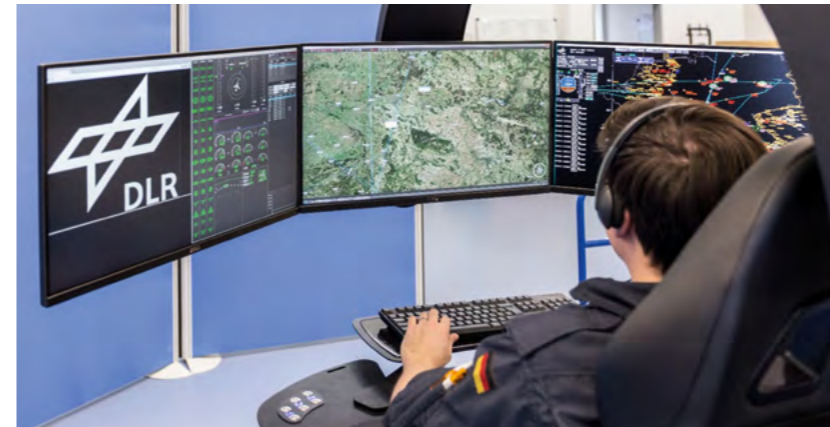
Unlike in manned aircraft, the pilot controls a HAP from the ground station. The remote pilot must rely on the aircraft's status information, course data and information from the civil airspace below.
