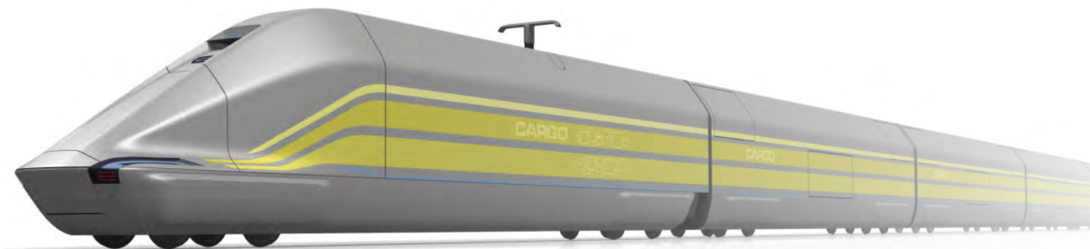
NGT CARGO power car with single wagon automatic coupler
