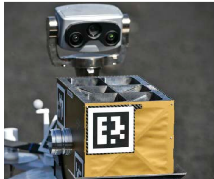
The black-and-white markings serve as name tags. The robots recognise each other and identify their payload. Here LRU2 is carrying a box to hold rock samples.
