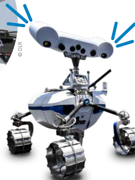
The final preparations at Base Camp on Mount Etna before robot LRU1 starts its mission. Several camera systems are mounted on its head. With the exterior filter wheels it recognises different frequency ranges.
