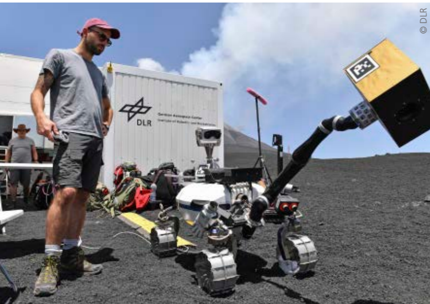
The LRU2 assistant uses its arm to perform analyses or handle payload boxes
