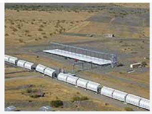
Fresnel reflectors and Parabolrinnen collectors in comparison
