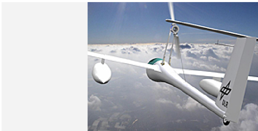
Antares: Research aircraft with self-launching fuel cell propulsion
