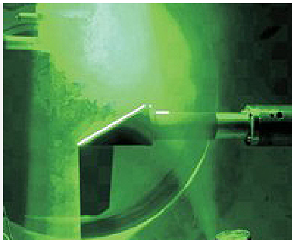
Wedge model inside the wind tunnel in Göttingen
