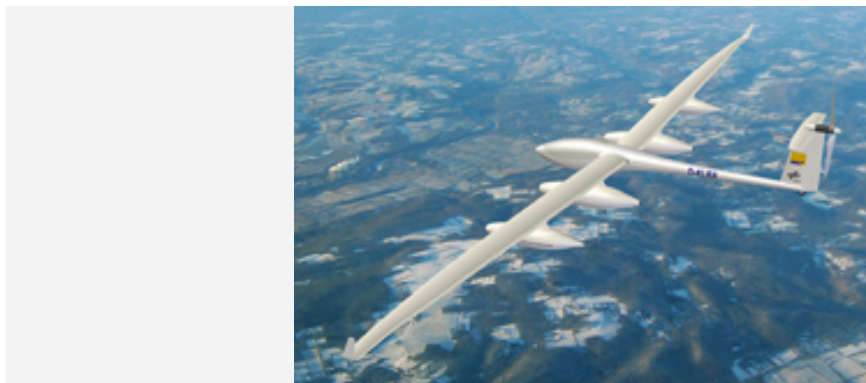
The Antares H3 – a next-generation fuel-cell powered aircraft
